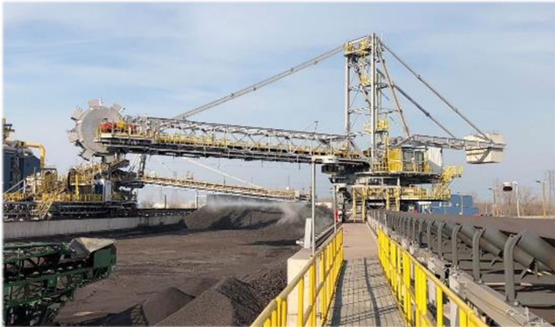
Pic.2: TAKRAF bucket-wheel reclaimer for handling HBI in the US can be seen in the foreground with stacker behind.
