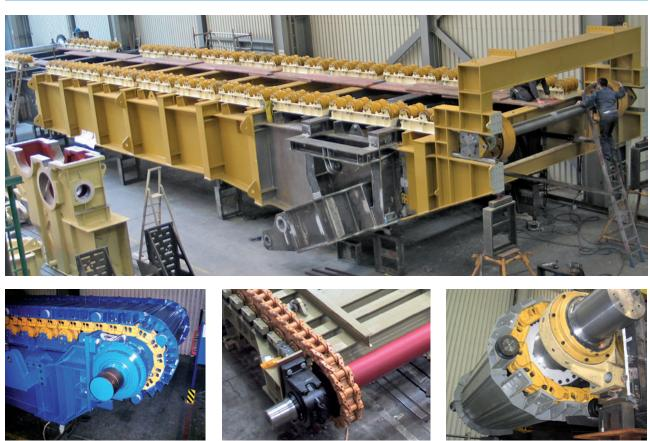
The apron feeders are available in outboard design with the chains outside the area in between the skirt boards preventing chains and rollers from falling spillage material and inboard design providing shorter and lighter pans. For outboard designs, return rollers are mounted at the pans or mounted underneath the pans as for inboard chains. If mounted at the pans, the rollers move on a rail. Pans are heavily reinforced. As appropriate, greased slide rails are mounted in full length.
